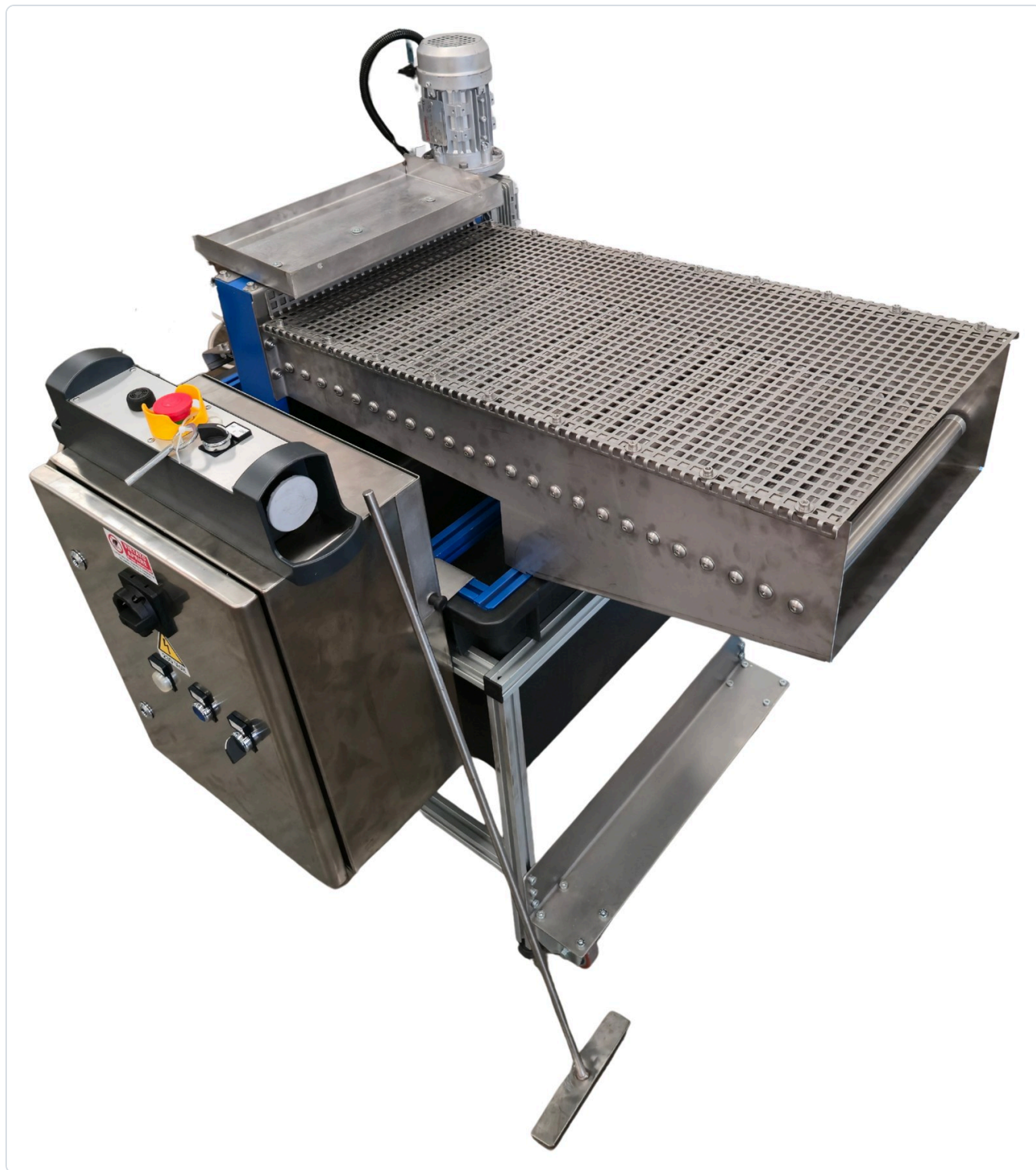
The loading mouth with idle rollers, the electrical panel with the controls and the collection tank below the wringing unit.
