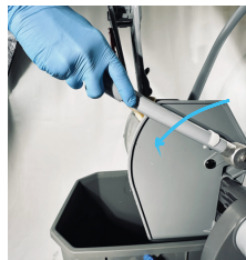
Figure 3 Squeezing the FoamFlex sponge
