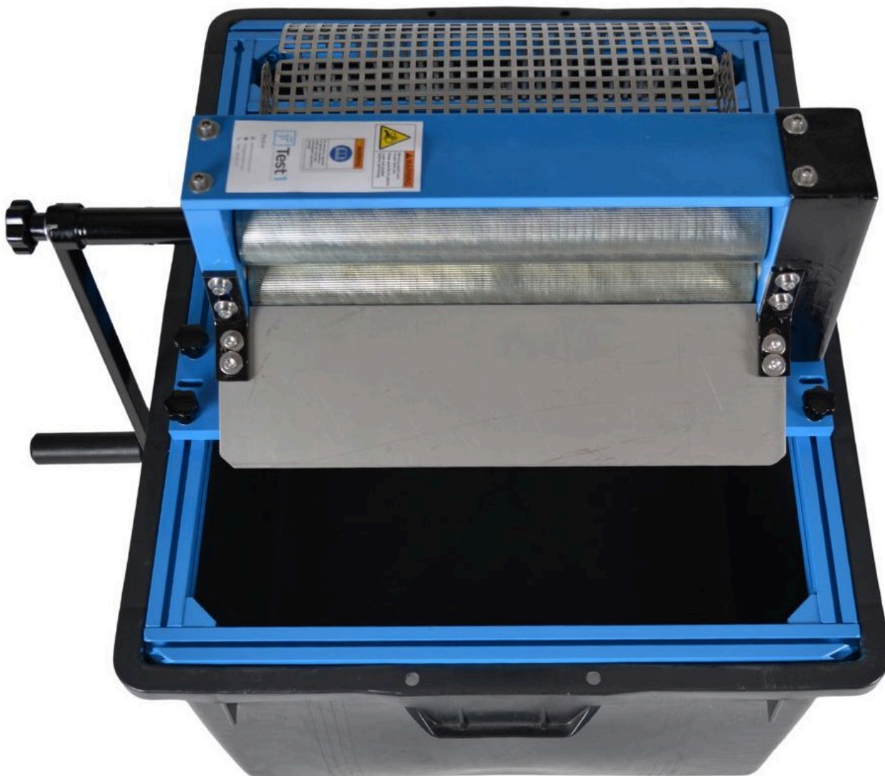
The wringing unit seen from above – opposing rollers, entry net, crank handle and collection tank below.
